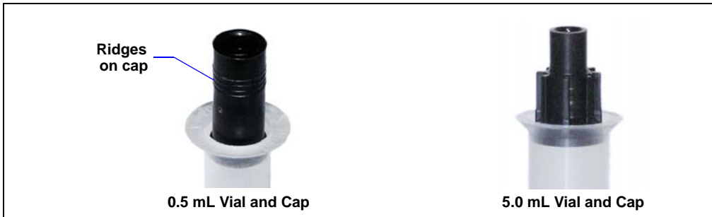
Figure 3-2. Caps Partially Inserted in Vials
