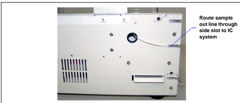
Figure B-2. Routing the Dionex AS-DV Sample Out Line to an IC System
